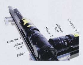
Figure 3.5: Collection optics for the helium line ratio diagnostic.
